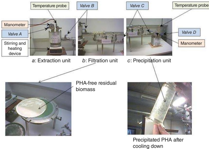
**Figure 6.6** Setup for extraction of PHAs from microbial biomass with acetone under high p/T conditions. Modified from [72].
