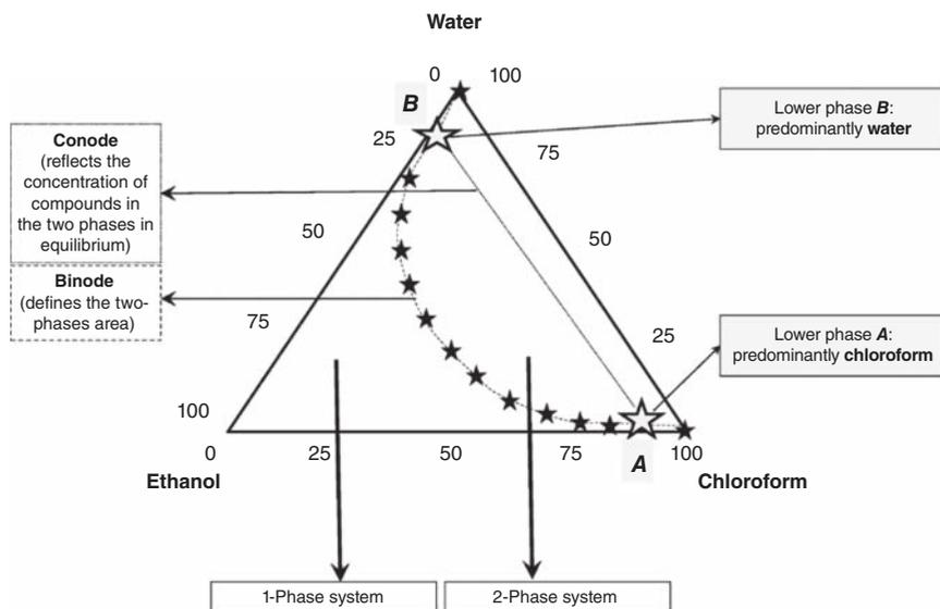
**Figure 6.5** One- and two-phase areas in the ternary system chloroform–ethanol–water. Source: Koller et al. [132]/with permission from Sciendo.
