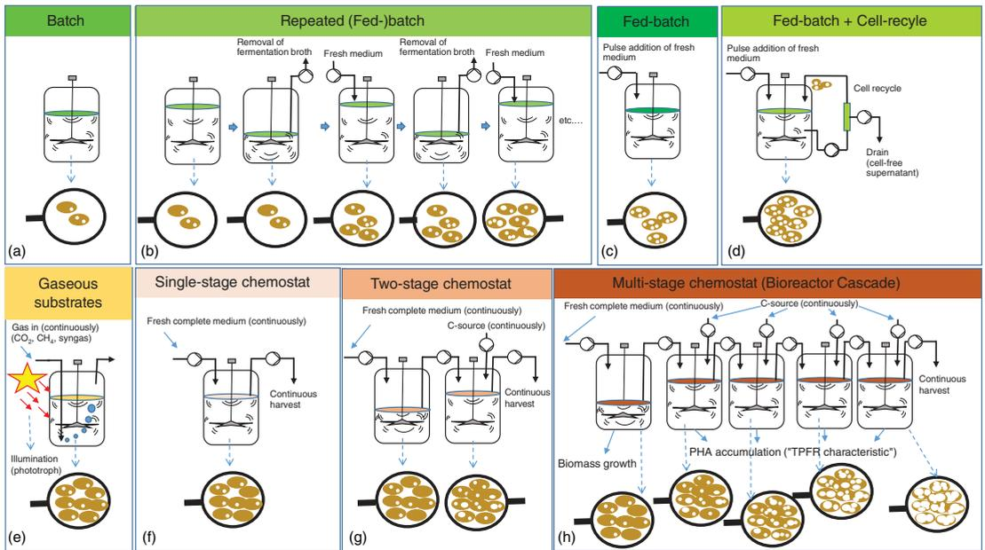
**Figure 6.3** Different operation strategies to run PHA production processes in bioreactors. (a) batch, (b) repeated (fed-) batch, (c): fed-batch, (d) fed-batch with cell-recycle, (e) gaseous substrates, (f) single-stage chemostat, (g) two-stage chemostat, (h) multi-stage chemostat (bioreactor cascade). Source: [111] Reproduced with permission of MDPI publishers, Basel.
