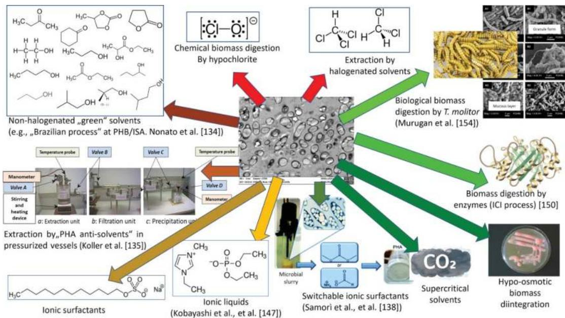
**Figure 6.4** Compilation of established and emerging PHA recovery methods by chemical and biological methods; coloration of arrows provides a rough, maybe preliminary, estimation of the overall sustainability of individual methods, with red being not or hardly sustainable and green indicating high sustainability. Source: Koller [130]/with permission from Sciendo.
