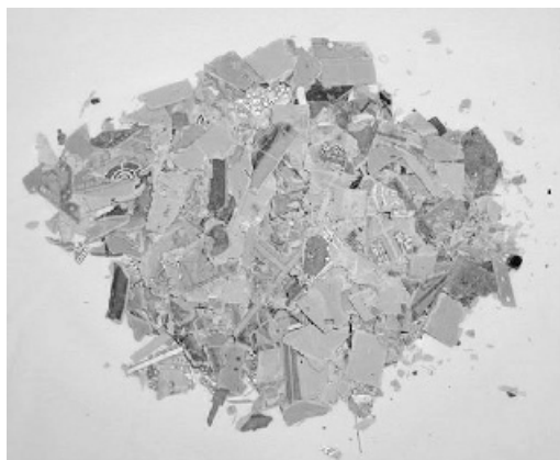
Figure 20.3 Nonpopulated computer circuit boards, pyrolysed at 350 and 450°C, 2 h at each stage and the corresponding residues. If necessary these residues can be sieved in fractions for accumulation of metals or used in total
