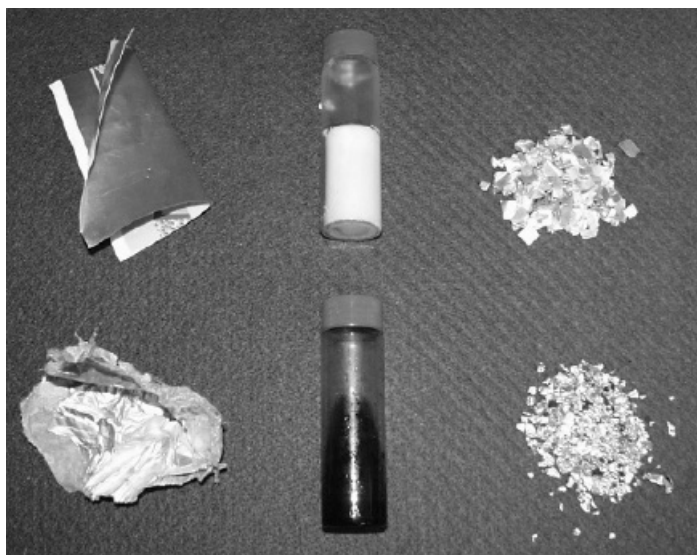
Figure 21.6 From left to right: original laminate, recovered condensable products and recovered aluminium. Top row, toothpaste tube laminate. Bottom row, depulped drink carton
