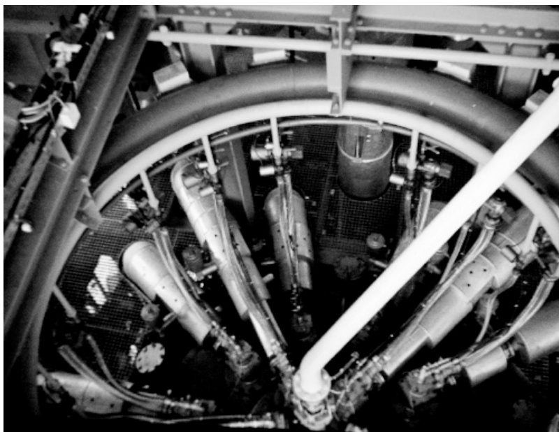
Figure 17.7 View of the top of the fluidized-bed reactor, DRP plant with the inlet of the 12 fire tubes
