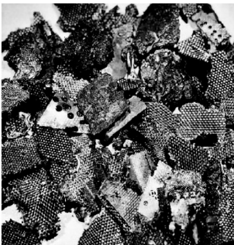
Figure 20.4 Populated computer circuit boards, pyrolysed at 350 and 450°C, 2 h at each stage and the related residues
