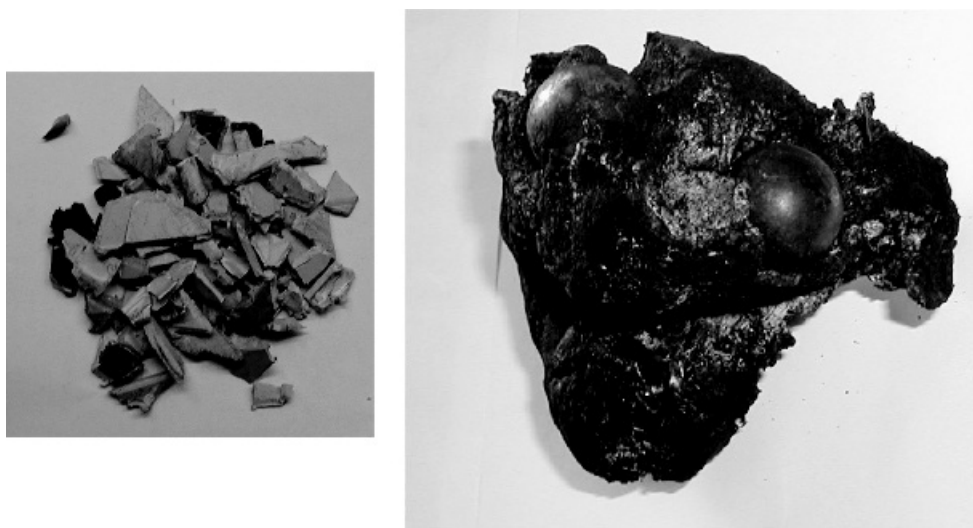
Figure 20.6 Housing fractions, pyrolysed at too low a temperature of about 350°C for 2 h, the residues becoming sticky
