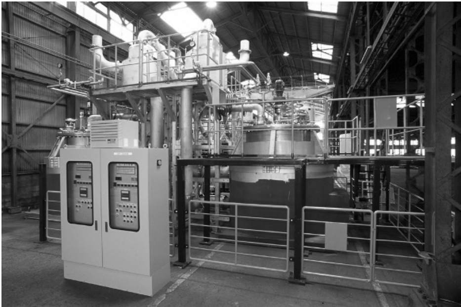
Figure 15.9 A commercial Thermofuel™ plant in Okinawa in Japan which processes agricultural plastics such as mulch and greehhouse films into diesel fuel to run green-house boilers for heating, tractors and other agricultural machinery. (Reproduced by permission of Ozmotech Pty Ltd)
