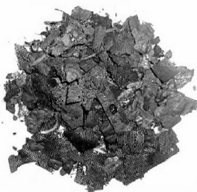
Figure 20.3 Nonpopulated computer circuit boards, pyrolysed at 350 and 450°C, 2 h at each stage and the corresponding residues. If necessary these residues can be sieved in fractions for accumulation of metals or used in total
