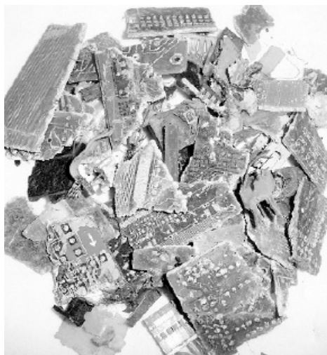
Figure 20.4 Populated computer circuit boards, pyrolysed at 350 and 450°C, 2 h at each stage and the related residues
