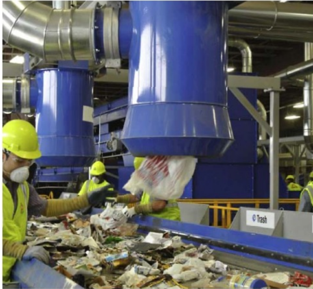
Figure 6.1 The FilmVac System [7]. Courtesy of Impact Air Systems.
