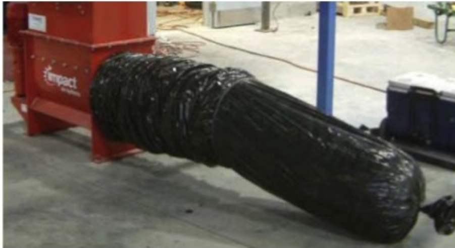
Figure 6.18 Sausage-like bale obtained by the Film Screw Compactor [25]. Courtesy of Impact Air Systems.
