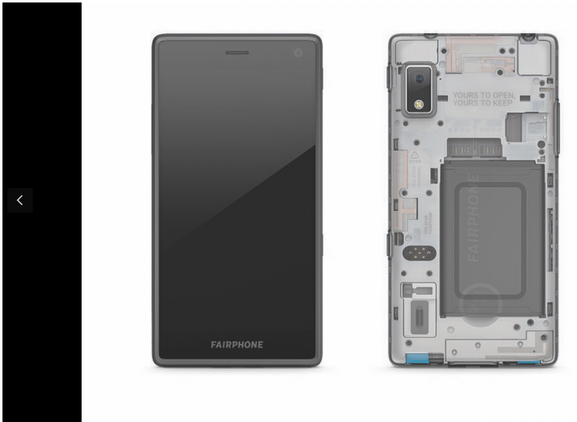
Front and back of a Fairphone 2 with a transparent case, showing the modular design. The individual components can be highlighted in the annotated image .
