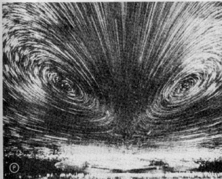
FIGURE 2.5-6. Velocity fields near a sudden contraction. The fluid moves from top to bottom in the photographs from a large reservoir into a small circular tube. (N) The streamlines in glycerin are straight and all directed toward the exit; (P) a 1.67% aqueous polyacrylamide solution shows a large toroidal vortex. [Photographs by H. Giesekus, given in A. B. Metzner, E. A. Uebler, and C. F. Chan Man Fong, AIChE J. , 15 , 750-758 (1969).]
