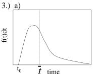
The initial observation is the shortest possible time to travel through the extruder, the time to travel along the rotations of the screw. Most of the material is not traveling this fast and the majority of the material runs through the extruder at t-bar in the plot. Some material remains in the extruder for a very long time since there is no-slip at the barrel wall.
