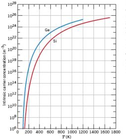
Figure 18.16 Intrinsic carrier concentration (logarithmic scale) as a function of temperature for germanium and silicon. (From C. D. Thurmond, "The Standard Thermodynamic Functions for the Formation of Electrons and Holes in Ge, Si, GaAs, and GaP," *Journal of The Electrochemical Society*, 122, [8], 1139 (1975). Reprinted by permission of The Electrochemical Society, Inc.)
