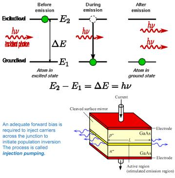
A schematic illustration of a GaAs homojunction laser diode. The cleaved surfaces act as reflecting mirrors.
