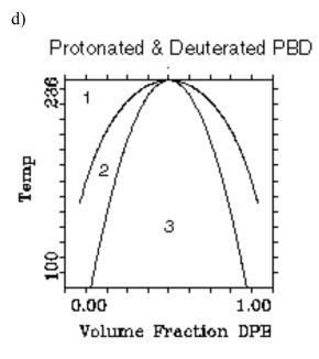
Figure 2. Upper critical solution temperature phase diagram. Regions 2 and 3 are 2-phase regimes, region 1 is the single phase regime. The line between region 2 and 1 is the cloud point curve or the binodal curve.
