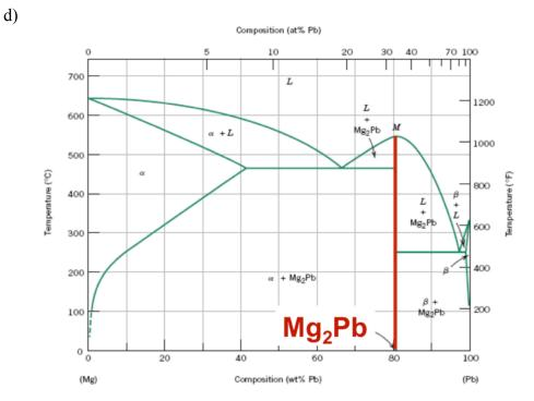
Note: intermetallic compound exists as a line - not an area – because stoichiometry (i.e. composition of a compound) is fixed.
