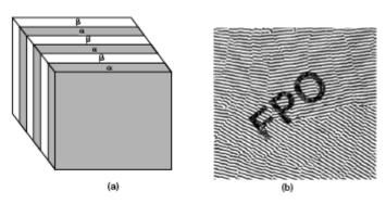
FIGURE 5.9. (a) Schematic representation of a lamellar or platelike microstructure as typically observed in eutectic alloys. (b) Photomicrograph of a eutectic alloy, 180× (CuAl<sub>2</sub>-Al). Reprinted with permission from *Metals Handbook*, 8th Edition, Vol. 8 (1973), ASM International, Materials Park, OH, Figure 3104, p. 156.
