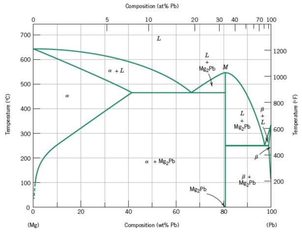
Figure 9.20 The magnesium-lead phase diagram. [Adapted from *Phase Diagrams of Binary Magnesium Alloys*, A. A. Nayeb-Hashemi and J. B. Clark (Editors), 1988. Reprinted by permission of ASM International, Materials Park, OH.]
