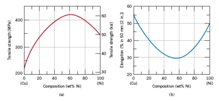
Figure 9.6 For the copper-nickel system, (a) tensile strength versus composition, and (b) ductility (%EL) versus composition at room temperature. A solid solution exists over all compositions for this system.
