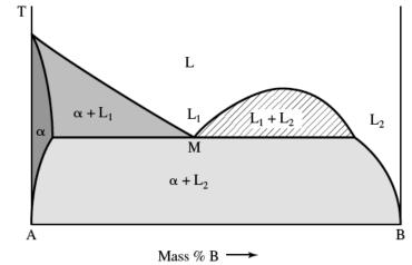
FIGURE 5.15. Schematic representation of a miscibility gap in the liquid state causing a monotectic reaction as given in Eq. (5.6).
