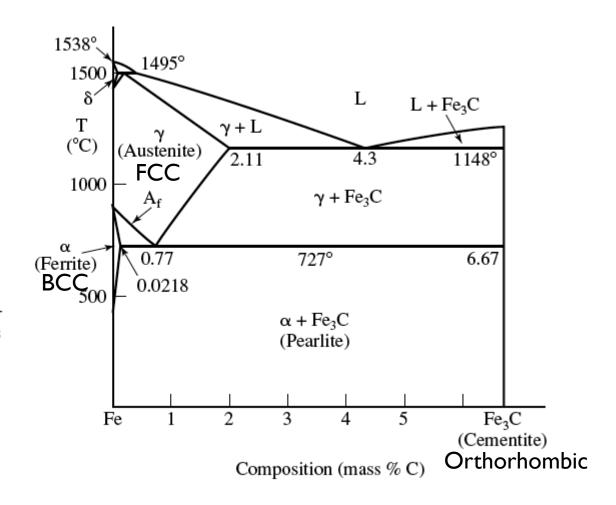
FIGURE 8.1. Portion of the iron–carbon phase diagram. (Actually, this section is known by the name *Fe*-*Fe*<sub>3</sub>*C phase diagram*.)  $A_f$  is the highest temperature at which ferrite can form. As before, the mass percent of solute addition is used (formerly called weight percent).
