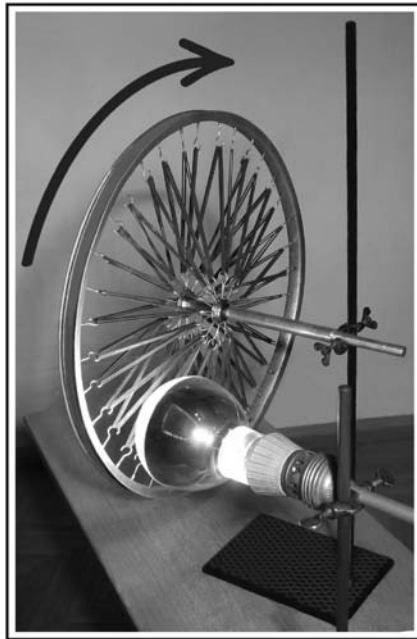
Fig. 7.9 An experiment to demonstrate the Guch–Joule effect. The device in this photo belongs to the lecture demonstration facility of Physics Department, Moscow State University; the image is courtesy of A.A. Aerov and S.B. Ryzhikov.
