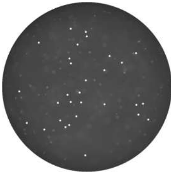
Fig. 4.7 An image in which the signal particles in the paraxial focus, have been masked out (indicated by white regions) to calculate the background noise. The vignetted area of the image has also been masked.
