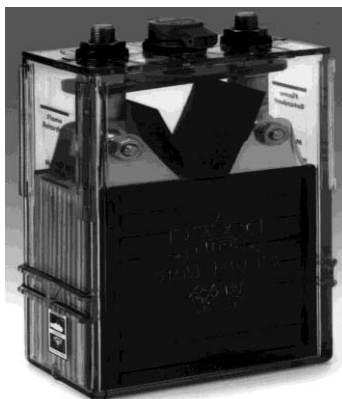
Figure 10-8 UDEL polysulfone is used for the transparent containers holding the potassium hydroxide electrolyte of a nickel–cadmium battery for electrical backup in railroad applications. The polysulfone container is unaffected by the alkaline electrolyte and is resistant to shock, vibration, and moisture. Courtesy of Solvay Advanced Polymers, L.L.C.
