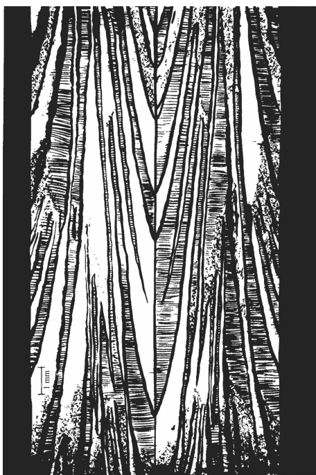
Figure 13.6 Matching fracture surfaces of a cleavage sample of poly(methyl methacrylate) showing colour alternation (green filter). (Reproduced from Berry, J.P. (1959) in Fracture (eds B.L. Auerbach et al.), John Wiley & Sons, New York, p. 263. Copyright (1959) John Wiley & Sons, Inc.)
