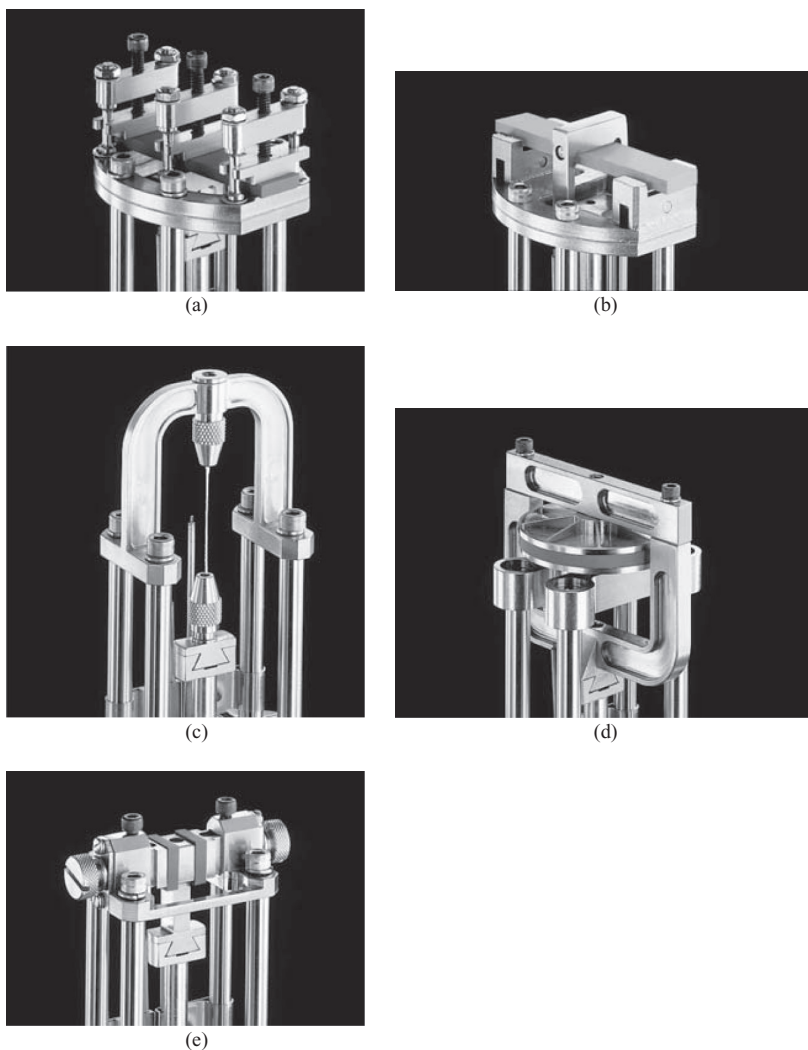
Figure 6.9 DMTA testing heads for various modes: (a) dual cantilever, (b) three-point bend, (c) tension, (d) compression and (e) shear sandwich (showing two specimens). Photographs by TA Instruments, Delaware USA. (Reproduced from Hillier, K.W. and Kolsky, H. (1949) An investigation of the dynamic elastic properties of some high polymers . Proc. Phys. Soc. B, 62 , 111. Copyright (1949) Institute of Physics.)
