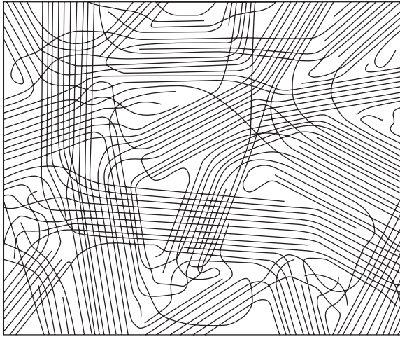
Figure 1.11 The fringed micelle representation of crystalline polymers. (Reprinted with permission from Hill, R. (ed.) (1953) Fibres from Synthetic Polymers , Elsevier, Amsterdam. Copyright (1953) Elsevier Ltd.)
