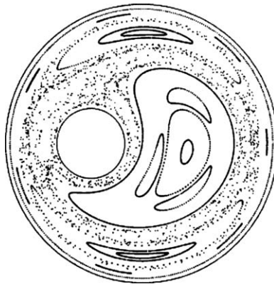
Fig. 7.10 Poincaré sections of viscous Newtonian flow in alternately turning eccentric cylinders. The inner cylinder turned counterclockwise for a given time, and then the outer cylinder was turned clockwise for 800 periods. There were 11 initial particles. [Reprinted by permission from J. Chaiken, R. Chevray, M. Tabor, and Q. M. Tan, "Experimental Study of Lagrangian Turbulence in Stokes Flow," Proc. R. Soc. London A , 408 , 165–174 (1986).]
