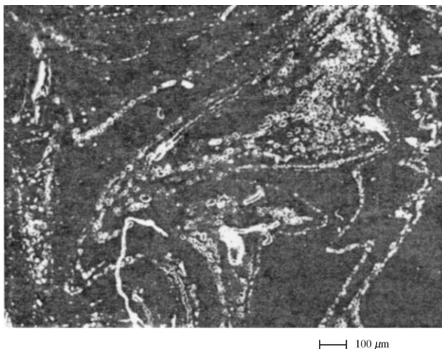
Fig. 11.33 Dispersed PS 685 streaks of ligaments and droplets in the equiviscous Blend 2. PS is flowing/deforming in an affine fashion in the expected stretching and folding pattern. Experiments were conducted at 180°C and 120 rpm. [Reprinted with permission from Proceedings of the Tenth Semi-annual Meeting of the Polymer Mixing Study , Polymer Processing Institute, Hoboken, NJ (1995).]
