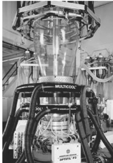
Fig. 14.13 (a) Schematic representation of the tubular blown film forming operation. (b) Photograph of a coextruded blown film die followed by blown film with external and internal cooling. [Courtesy of Windmoeller & Hoelscher (Lincoln RI).]
