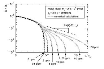
**FIG. 8.** Numerical calculations of the diameter  $D/D_0$  as a function of the reduced time  $t/\tau_0$  for a dilution series of polystyrene in styrene oligomer. Even though the longest relaxation time  $\tau_0$  is held *constant* for all calculations, only the calculations for the highest concentrations show a profile in accordance with the indicated slope of exp( $-t/3\tau_0$ ) of Eq. (22).
