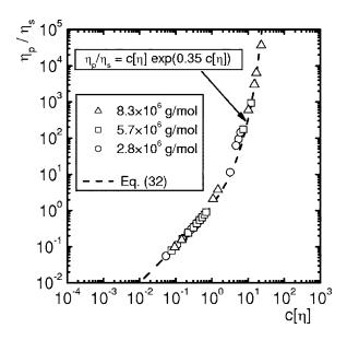
**FIG. 13.** Specific viscosity  $\eta_p/\eta_s$  as a function of the reduced concentration  $c[\eta]$  for solutions of polystyrene in DEP, determined with capillary viscometric measurements at lower concentrations, and cone-and-plate shear rheometry at higher concentrations. The continuous line gives the best fit to the structure-property relationship of Eq. (32).
