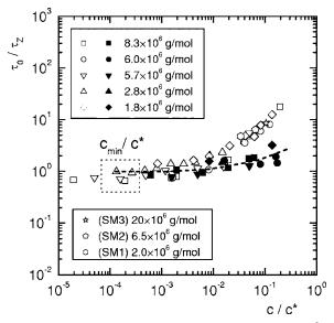
**FIG. 11.** Reduced relaxation times  $\tau_0/\tau_z$  as a function of the reduced concentration  $c/c^*$ , obtained from best fits of the numerically calculated diameter evolution to the experiments presented in Fig. 2 with  $\tau_0$  as an adjustable parameter (hollow symbols). For comparison, also the results from the SAOS experiments in Fig. 7 are given (filled symbols). Also the range of critical concentrations  $c_{\min}/c^*$  for the different molar masses is indicated by the rectangle.
