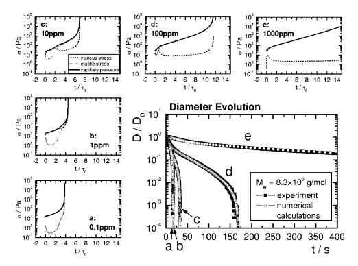
**FIG. 10.** Comparison of the numerically calculated diameter evolution with experimental observations for a dilution series of a Boger fluid with a molar mass  $M_w = 8.3 \times 10^6$  g/mol. The initial diameters for the numerical calculations were taken from the experimental observations. In addition, the calculated stress distribution is given for each concentration. The critical concentration from Eq. (41) is  $c_{\min}=0.36$  ppm.
