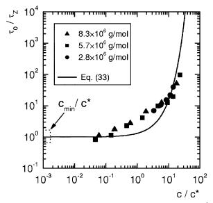
**FIG. 12.** Reduced relaxation times  $\tau_0/\tau_z$  as a function of the reduced concentration  $c/c^*$  for dilution series of polystyrene in DEP. In addition, the theoretical concentration dependence of the relaxation time according to Eq. (33) is shown. Also the range of critical concentrations  $c_{\min}/c^*$  for the different molar masses is indicated by the rectangle.
