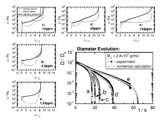
**FIG. 9.** Comparison of the numerically calculated diameter evolution with experimental observations for a dilution series of a polystyrene Boger fluid with a molar mass  $M_w = 2.8 \times 10^6$  g/mol. The initial diameters for the numerical calculations were taken from the experimental observations. In addition, the calculated evolution in stress distribution is given for each concentration. The critical concentration from Eq. (41) is  $c_{\min} = 1.7$  ppm.
