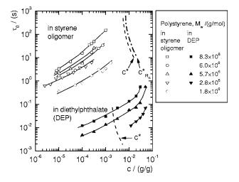
**FIG. 3.** Relaxation time  $\tau_0$  as a function of the concentration *c*, determined by regression of the experimental data in the exponential decaying regime of Figs. 2 and 14 to Eq. (22). The dashed lines map the variation of relaxation time  $\tau_0$  with critical concentrations  $c^*$ . These values were determined by extrapolating the observed trends of relaxation times to the critical values determined from Eqs. (1) and (27).
