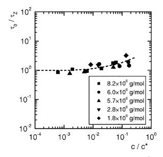
**FIG. 5.** Reduced relaxation time  $\tau_0/\tau_z$  as a function of the reduced concentration  $c/c^*$ , determined from SAOS experiments and fits of the moduli to Eqs. (2) and (3) for polystyrene of different molar masses dissolved in styrene oligomer.
