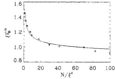
**Figure 3.**  $\xi l_B^{1/3}$  as a function of  $N/\xi^2$  for unscreened chains. Different symbols represent Barrat and Boyer's simulation data with different  $N$  (asterisk,  $N = 50$ ; triangle,  $N = 100$ ; diamond,  $N = 200$ ; square,  $N = 400$ ). The solid line is a two-parameter fit using eq 2.6.
