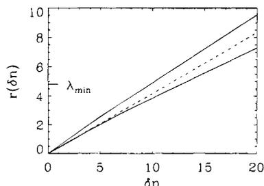
**Figure 4.** Direct distance  $r(\delta n)$  as a function of monomer separation  $\delta n$  calculated using eq 2.28. The two solid lines are for  $\kappa^{-1} = \infty$  (upper curve) and  $\kappa^{-1} = 20$  (lower curve). The dashed line is a straight line extrapolated from the initial slope of the curve for the screened case.  $\lambda_{\min}$  marks the cutoff wavelength. All the lengths are measured in units of  $a$ .
