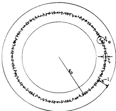
**Figure 1.** Schematic diagram of the base state, where the chain forms a circular loop with radius  $r_0$  and core size  $\xi$ .
