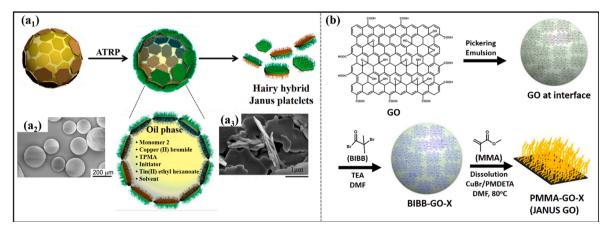
**Fig. 4.** (a<sub>1</sub>) Schematic synthesis of Janus platelet of Kaolinite/polymer composite, (a<sub>2</sub>) SEM images of the wax sphere with the Br modified Kaolinite and (a<sub>3</sub>) the Janus platelet with two polymers at the opposite sides. Adapted with permission from Ref. [65]. Copyright 2014 American Chemical Society. (b) Schematic synthesis of the Janus platelet of PMMA-GO-X. Adapted with permission from Ref. [67]. Copyright 2017 American Chemical Society.
