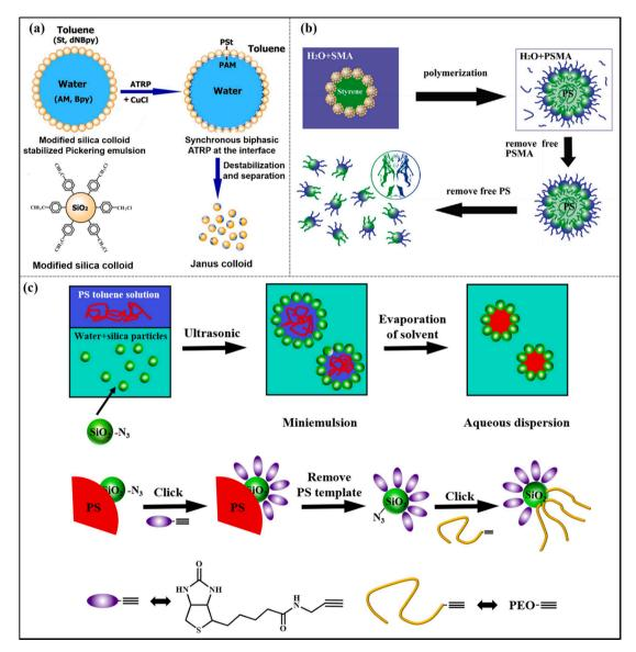
**Fig. 3.** (a) Janus particle by the synchronous biphasic ATRP grafting at a Pickering emulsion interface. Adapted with permission from Ref. [58]. Copyright 2008 Wiley. (b) Janus silica particle by surface-initiated free radical polymerization at a Pickering emulsion interface. Adapted with permission from Ref. [59]. Copyright 2009, American Chemical Society. (c) Bio-conjugated Janus particle by click reaction. Adapted with permission [60]. Copyright 2009 American Chemical Society.
