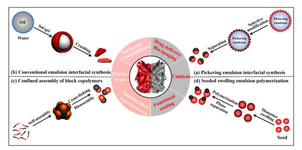
Fig. 1. Representative synthetic approaches to Janus polymer/inorganic nanocomposites and the representative performances. (a) Pickering emulsion interfacial synthesis. (b) Conventional emulsion interfacial synthesis. (c) Confined self-assembly of block copolymers. (d) Seeded swelling emulsion polymerization.
