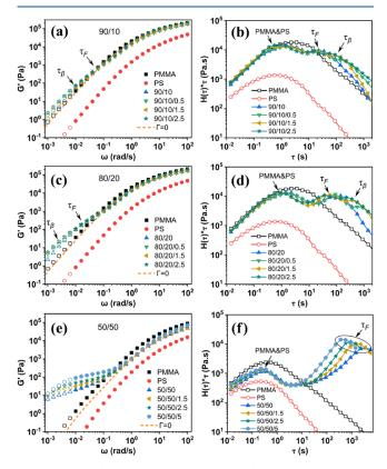
**Figure 9.** (a,c,e) Storage moduli and (b,d,f) relaxation spectra of PMMA/PS 90/10 and 80/20 blends at 200 °C and 50/50 blends at 220 °C with various JNPs amounts. The solid symbols are the results from dynamic tests, and the hollow symbols are the conversion data from creep tests. The dashed line is the contribution of the blend components at  $\Gamma=0$  based on Kerner's model (eq 4).
