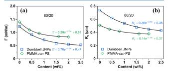
**Figure 8.**  $\Gamma$  and  $R_{\nu}$  of PMMA/PS 80/20 blends as a function of JNPs and PMMA-*ran*-PS concentration. The results for PMMA-*ran*-PS are extracted from ref 62. The lines are the fitting result of eqs 5 and 8.
