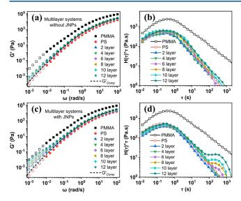
**Figure 12.** Frequency dependence of G' (a,c) and weighted relaxation time spectra (b,d) of multilayer systems with various layer numbers in the absence (a,b) and in the presence of JNPs ( $\Sigma = 16.4\%$ ) (c,d) at 220 °C. The dashed line is the total contribution of the neat components based on eq 11.
