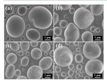
**Figure 5.** High-magnification SEM micrographs of some particularly selected large droplets to show the localization of JNPs based on 80/20 blends after the frequency sweep test and PS phase etching with various JNPs concentrations: (a) 0%, (b) 1%, (c) 2%, and (d) 2.5%.
