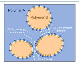
**Figure 1.** Schematic illustration of the Marangoni stress induced by JNPs located at the interface between both phases in a blend.
