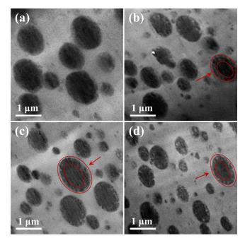
**Figure 6.** TEM images of PMMA/PS (80/20) blends after the frequency sweep test with various JNP concentrations: (a) 0%, (b) 1%, (c) 2%, and (d) 2.5%. The red lines are to guide the eye.
