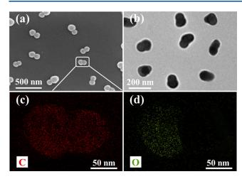
Figure 3. (a) SEM and (b) TEM images of dumbbell-shaped PMMA-PS JNPs; SEM-EDS elemental maps of (c) C and (d) O of a single JNP based on (a).
