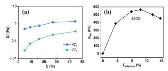
**Figure 14.** (a) Dependence of  $G_5'$  and  $G_6'$  on  $\Sigma$  for 12-layered samples with JNPs at 220 °C; (b) variation of Marangoni stress ( $\sigma_{\rm Ma}$ ) with effective interfacial coverage ( $\Sigma_{\rm effective}$ ) of JNPs for 80/20 blends at 200 °C.
