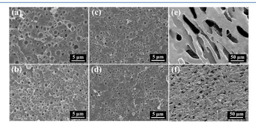
Figure 4. SEM micrographs of (a) 80/20, (b) 80/20/1, (c) 80/20/2, (d) 80/20/2.5, (e) 50/50, and (f) 50/50/5 blends after etching PS.
