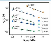
**Figure 10.** JNP concentration  $(w_{\rm JNPs})$  dependence of relaxation times  $\tau_{\rm F}$  and  $\tau_{\beta}$  for 50/50, 80/20, and 90/10 blends. The solid line corresponds to the linear regression of eq 10.
