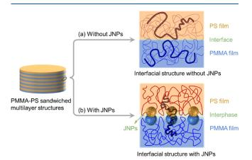
Figure 2. Schematic illustration of the interface between sandwiched multilayer structures (a) without and (b) with JNPs.
