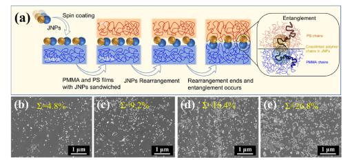
Figure 11. (a) Schematic illustration of the annealing rearrangement of JNPs at the PMMA/PS interface and subsequent penetration and entanglement with the bulk phases. (b–e) SEM images of JNP distributions at the interface of a PMMA/PS multilayer observed after a frequency sweep test at 220 °C with the PS films removed via selective etching. The feeding JNP concentration in the spin-coating solution was varied: (b) 0.1 wt %, (c) 0.3 wt %, (d) 1 wt %, and (e) 3 wt %.
