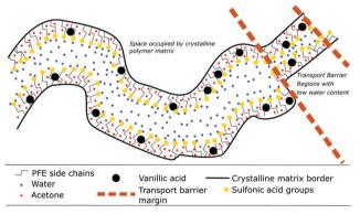
Fig. 6 Schematic presentation of the microscopic structure of Nafion with the preferred locations of water, acetone, and vanillic acid.
