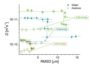
Fig. 2 Dependence of the measured self-diffusivities of acetone (stars) and water (squares) on root MSD in VA-functionalized Nafion membranes at 296 K. Water concentration in Nafion was held constant at  $\sim$ 2 mmol g<sup>-1</sup>. Solid lines are guidelines shown as visual aids.
