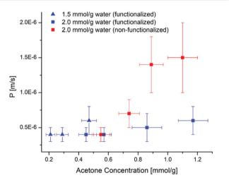
Fig. 3 Estimated values for domain boundary permeance for water with changing acetone concentration at 1.5 mmol  $\ensuremath{\mathrm{g}^{-1}}$  water (blue triangles) and 2 mmol  $g^{-1}$  water (blue and red squares). Red points indicate values of P estimated for non-functionalized Nafion membranes, 19 while blue points indicate P estimates for Nafion functionalized with VA
