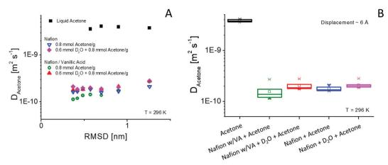
Fig. 7 Acetone self-diffusion coefficients from QENS measurements presented as a function of RMSD (A), and acetone self-diffusion coefficients averaged for the full QENS range (B). Each box in (B) represents one standard deviation with the internal line denoting the mean, open symbols represent the mode, the 'x' symbols denote the extremes
