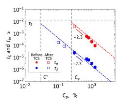
**FIG. 8.** (Color online) Characteristic lengths  $\xi$ , a (left) and characteristic times  $\tau_{\xi}$ ,  $\tau_{e}$  (right) as a function of polymer concentration on the log-log scale. Filled circles show these quantities estimated from the original MSD curves before performing the TCS (Fig. 7 left), whereas open squares represent those obtained from the MSD master curve after the TCS (Fig. 7 right).
