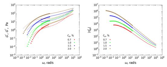
FIG. 5. (Color online) Left: Dynamic moduli of PEO aqueous solutions. Solid (or dashed) lines: storage (or loss) modulus by micro-rheology. Closed (or open) circles: storage (or loss) modulus by macro-rheology. Polymer concentrations are 0.7% (red), 1.0% (green), 1.5% (blue), and 2.0% (brown). Right: Absolute value of the complex specific viscosity of PEO aqueous solution. Solid lines: micro-rheology. Closed circles: macro-rheology. Probe concentration is 0.25% for all polymer concentrations.
