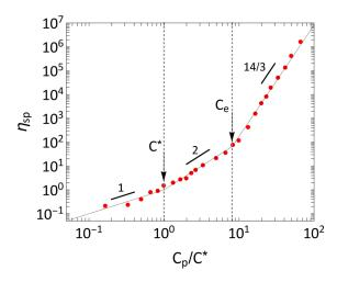
**FIG. 2.** Specific viscosity of PEO aqueous solution measured by macrorheology as a function of PEO concentration  $C_p$ . The overlap concentration is  $C^* = 0.030\%$ , and the entanglement concentration is  $C_c = 0.25\%$ .
