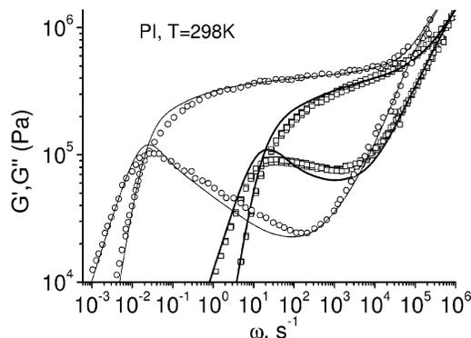
**Figure 16.** Linear rheology data for polyisoprene of  $M_w = 75$  K from ref 24 (squares) and of  $M_w = 500$  K from ref 25 (circles). Squares are fitted by slip-links model, and circles, by analytical model.
