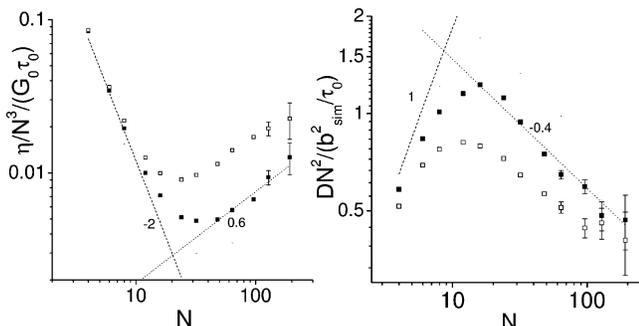
**Figure 5.** Normalized viscosity (a) and self-diffusion coefficient (b) predictions with and without constraint release (filled and open symbols correspondingly). Rouse model predictions are shown by dotted lines,  $-0.4$  and  $0.6$  slopes by dashed lines.
