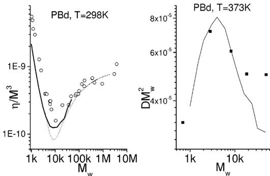
**Figure 19.** Normalized viscosity and self-diffusion data for polybutadiene as a function of molecular weight. Viscosities are from ref 28, diffusion from ref 22. Solid lines are predictions by the model, with parameters obtained from the fit of linear rheology data; dotted line: predictions of our earlier analytical theory.<sup>19</sup>
