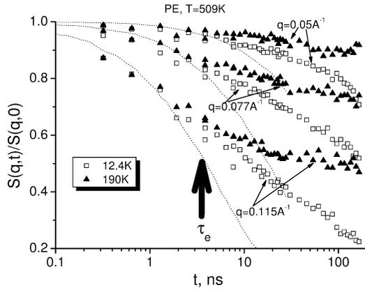
**Figure 1.** Normalized dynamic structure factor as measured by NSE<sup>14</sup> for two different molecular weights of PEB-2 at three different  $q$ -vectors. Dotted lines are predictions of the Rouse theory.
