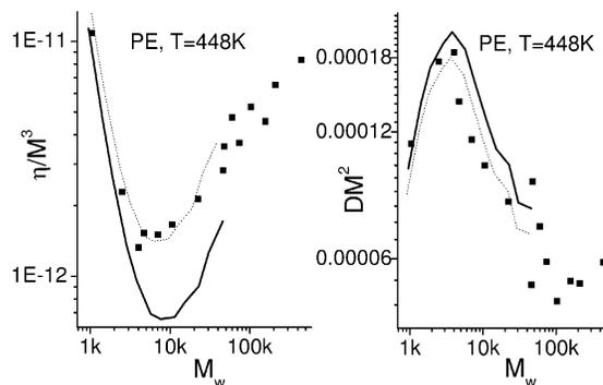
**Figure 12.** Normalized viscosity and diffusion coefficient compared with the data of ref 18. Solid lines: predictions using parameters from NSE; dotted lines: best fits using  $M_0$  as fitting parameter.
