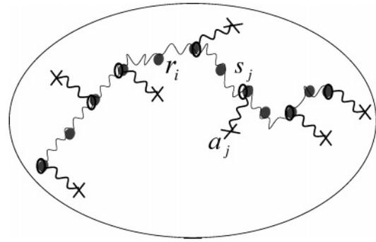
**Figure 3.** Slip-links model of entangled polymer chain. Spheres connected by the thin springs represent a standard Rouse chain, thick springs are additional potentials, attached to slip-links on a chain  $\mathbf{s}_j$  and to fixed anchoring points  $\mathbf{a}_j$  (crosses).
