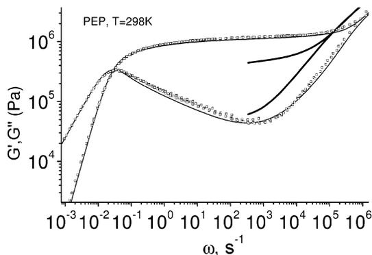
**Figure 14.** Linear rheology of the same PEP sample as used in ref 15. Solid lines: predictions with parameters obtained from NSE; dotted lines: best fits by the model. Only the high-frequency region can be compared.
