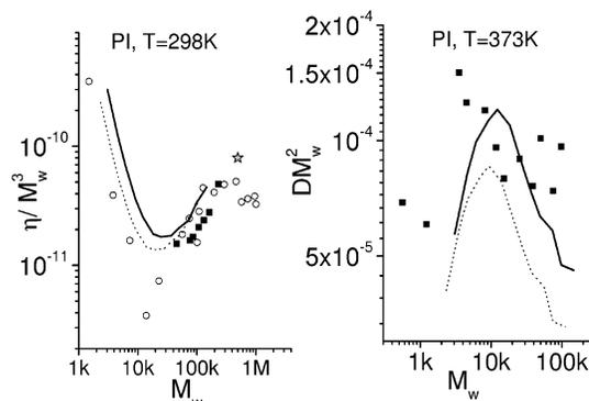
**Figure 17.** Normalized viscosity and self-diffusion data for polyisoprene as a function of molecular weight. Viscosities are from ref 23 (squares), ref 24 (circles), and ref 25 (star); diffusion from ref 22. Solid lines are predictions by the model using linear rheology from ref 25, dotted lines from ref 24.
