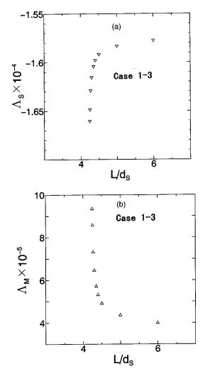
FIG. 11. Relation between  $\Lambda_i$  (*i*=S,M) and the surface separation *L* in case 1-3: *i*=S (a) and *i*=M (b). In case 1-3, both the surface and the solute are solvophobic.
