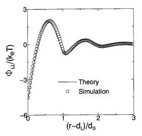
FIG. 1. Interaction between large hard spheres theoretically calculated using method 3 ( $d_L/d_s=10$  and  $\eta_s=0.314$ ). The force obtained in the computer simulation of Biben *et al.* (Ref. 34) was smoothed and integrated by Roth *et al.* (Ref. 7), yielding the simulation data compared with the theoretical result.
