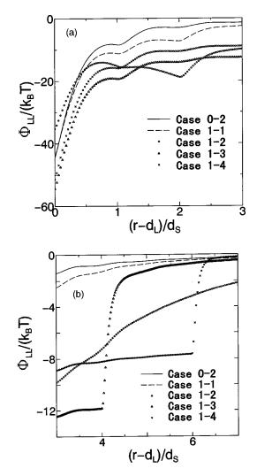
FIG. 3. Interaction between solvophobic surfaces immersed in solvent–solute mixture:  $0 \le (r - d_L)/d_S \le 3$  (a) and  $3 \le (r - d_L)/d_S \le 7$  (b). The solute has considerably high solvophobicity. See Table II for the definition of cases 1-1, 1-2, 1-3, and 1-4. In case 0-2, no solute is added to the solvent.
