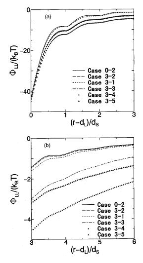
FIG. 5. Interaction between solvophobic surfaces immersed in solvent–solute mixture:  $0 \le (r-d_L)/d_S \le 3$  (a) and  $3 \le (r-d_L)/d_S \le 6$  (b). The solute has considerably high solvophilicity. See Table IV for the definition of cases 3-1, 3-2, 3-3, 3-4, and 3-5. In case 0-2, no solute is added to the solvent.
