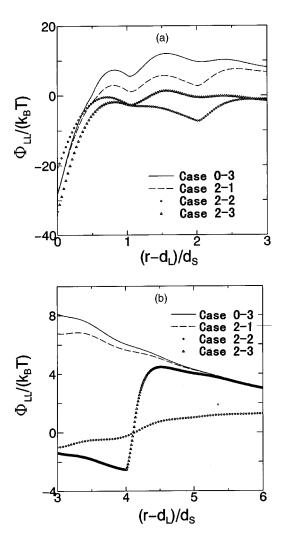
FIG. 4. Interaction between solvophilic surfaces immersed in solvent–solute mixture:  $0 \le (r-d_L)/d_S \le 3$  (a) and  $3 \le (r-d_L)/d_S \le 6$  (b). The solute has considerably high solvophobicity. See Table III for the definition of cases 2-1, 2-2, and 2-3. In case 0-3, no solute is added to the solvent.
