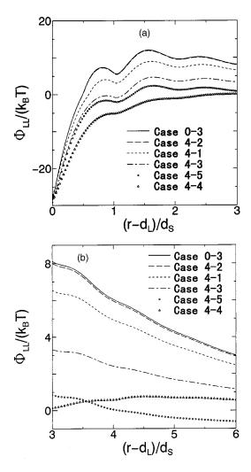
FIG. 6. Interaction between solvophilic surfaces immersed in solvent–solute mixture:  $0 \le (r-d_L)/d_S \le 3$  (a) and  $3 \le (r-d_L)/d_S \le 6$  (b). The solute has considerably high solvophilicity. See Table V for the definition of cases 4-1, 4-2, 4-3, 4-4, and 4-5. In case 0-3, no solute is added to the solvent.
