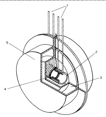
FIG. 4. Calorimetric block of the capillary scanning microcalorimeter DASM-4. (1) Capillary inlets; (2) helical capillary cell with heater; (3) internal shell; (4) thermopile measuring the temperature difference between the capillary cells; (5) external shell.
