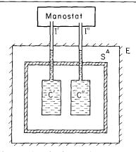
FIG. 2. Undismountable calorimetric block with the cells completely filled with liquid samples through the capillary inlets 1' and I". The measuring volume of the cells is fixed by the point at which the adiabatic shell (S) contacts with the capillary inlet and shunts the difference heat effect. The manostat is used to apply extra pressure on the liquid for squeezing the bubbles which might be left in the cells and for preventing their appearance upon heating.
