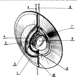
FIG. 3. Calorimetric block of the scanning microcalorimeter DASM-1M. (1,2) Internal and external adiabatic shells with heaters; (3) calorimetric cells; (4) shell thermosensor; (5, 6) capillary inlets; (7) thermopile; (8) cell heater; (9) internal shield rim; (10) external shield rim.
