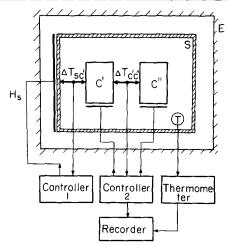
FIG. 1. Differential adiabatic scanning calorimeter with two identical cells (C' and C'') heated at a constant rate and a controlled temperature of the surrounding shell (S).
