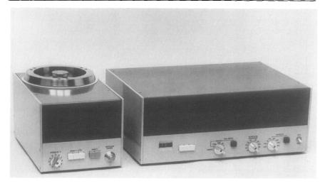
FIG. 5. Capillary scanning microcalorimeter DASM-4, manufactured by the Bureau of Biological Instrumentation of the Academy of Sciences of the USSR.
