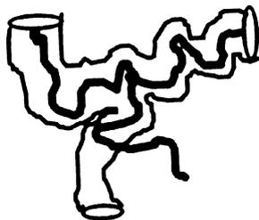
**Fig. 6.** Proposed mechanism of entangled dynamics of a star polymer in a melt. Retractions as shown partially renew the tube, beginning with rapid retractions near the free end and much more rarely renewing deeper parts of the molecule
