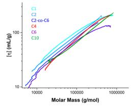
Figure 5. Mark-Houwink plot of LLDPEs measured by SEC (THF, 35°C).
