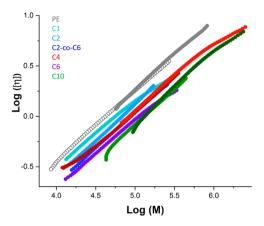
**Figure 3.** Mark—Houwink plots of LLDPEs measured by HT-SEC. The open circles are the intrinsic viscosity data measured for NIST SRM 1475A, for reference.
