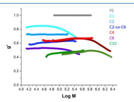
**Figure 4.** Viscometric contraction factor, g', across the molar mass distribution for the model LLDPEs studied. g' = 1 for linear polyethylene.
