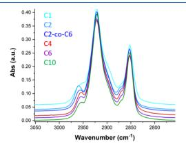
**Figure 2.** ATR-FTIR measurements of model LLDPEs in this study across the alkyl CH stretching region relevant to HT-SEC with IR detection. The total area of the alkyl region (2800–3000 cm<sup>-1</sup>) has been normalized between the spectra for comparison. Note the shift in the methyl asymmetric stretch centered near 2950 cm<sup>-1</sup> for each branch length.
