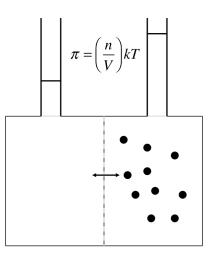
2) The Figure above shows a model for an osmotic pressure measurement.
