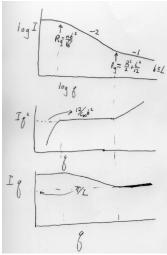
4)  $R_g^2$  for the chain =  $N_K 2l_{per}^2/3$ . The plot yields  $R_g$  and  $l_{per}$  so  $N_K$  can be determined.  $/l_{per}$  is the intercept of the modified Kratky plot or can be obtained from  $R_g$  for the persistence transition using the function obtained in question 1.
