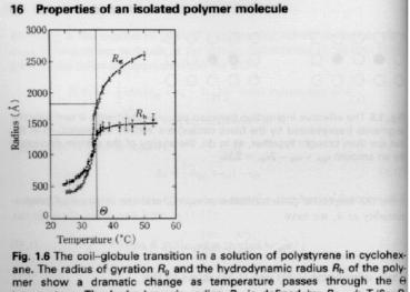
ane. The radius of gyration  $R_g$  and the hydrodynamic radius  $R_h$  of the polymer show a dramatic change as temperature passes through the  $\theta$  temperature. The hydrodynamic radius  $R_h$  is defined by  $R_h = k_B T/6\pi\eta D$ , where D is the diffusion constant of the polymer and  $\eta$  is the viscosity of the solvent. (Sun, S.T., Nishio, I., Swislow, G., and Tanaka, T. (1980). J. Chem. Phys., 73, 5971, Fig.2.)
