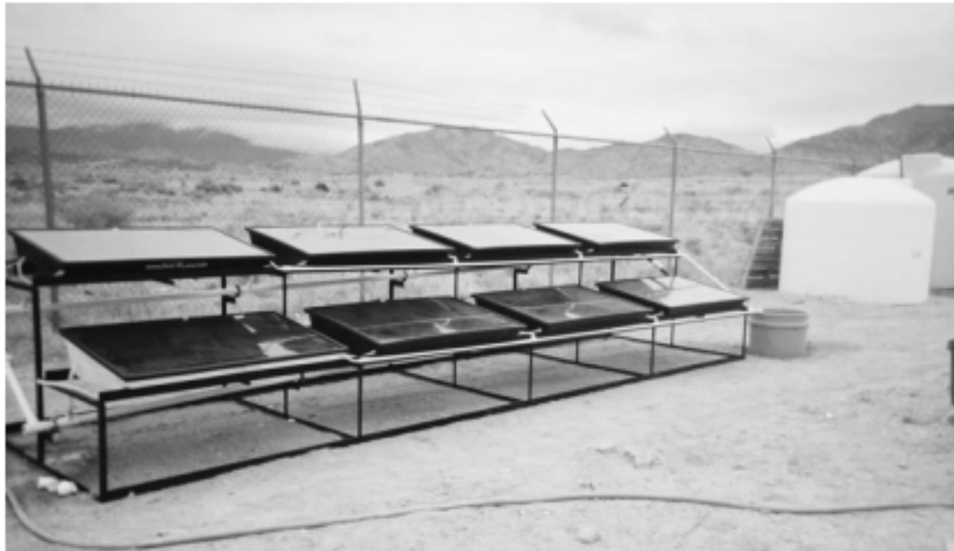
FIGURE 4.28 SolAqua solar still village array under test at Sandia National Laboratories.
