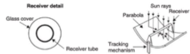
FIGURE 3.13 Schematic of a parabolic trough collector.
