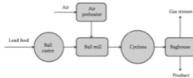
FIGURE 7.9 Flowchart of Ball mill process.
