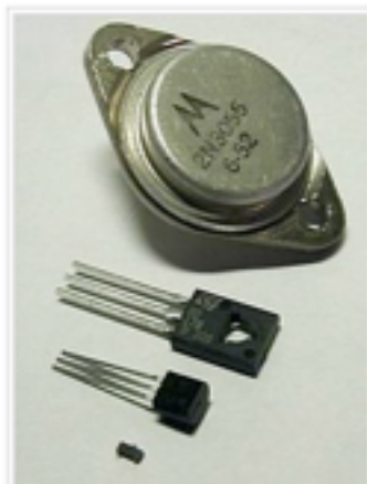
Assorted discrete transistors. Packages in order from top to bottom: TO-3, TO-18, TO-18, SOT-23
