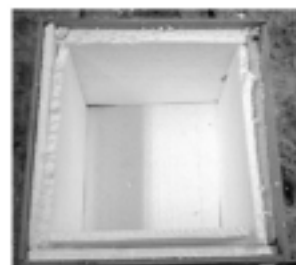
Figure 6-7 The box lined with polystyrene.
