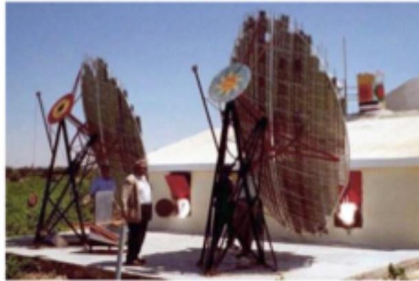
Figure V.i.4 Scheffeler solar community collector [19]
