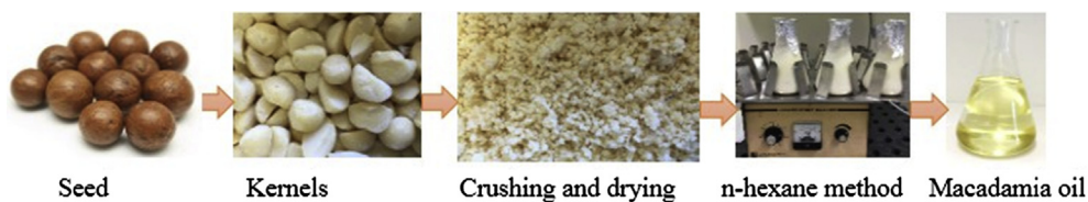
Figure 13.3 Oil extraction by n-hexane method from macadamia seed.
