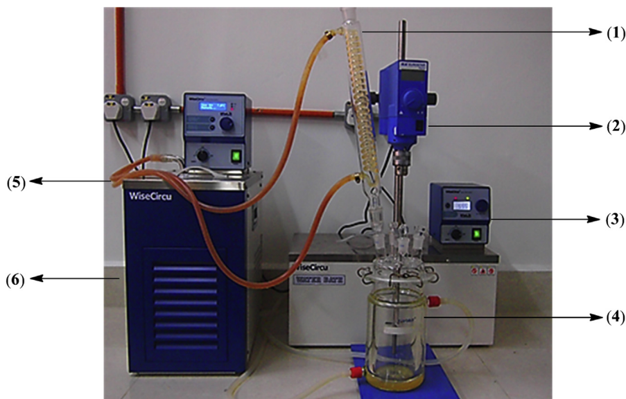
Figure 17.4 Experimental setup used to perform biodiesel production: (1) reflux condenser, (2) overhead mechanical stirrer, (3) circulating water bath, (4) jacketed glass batch tank reactor (1 L), (5) hoses, and (6) refrigerator [1].
