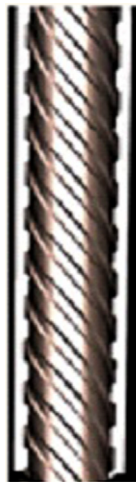
Figure 2.28 Spiral water tubes. Source: ALSTOM Presentation to The Kuljian Corporation, Philadelphia. August 25, 2010.
