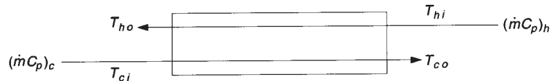
Figure 3.17.1 Schematic of an adiabatic counterflow heat exchanger showing temperatures and capacitance rates of the hot and cold fluids.
