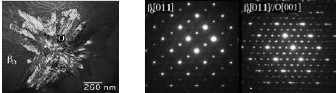
Figure 5. Electron diffraction used to determine orientation relationship of the Ti_2AlNb (O) phase precipitate in Nb solid-solution ( ).
