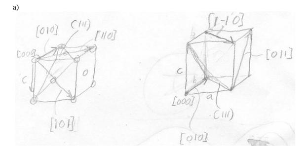
b) (111) is a hexagonal plane in the FCC structure. These planes stack in an ABCABC... motif in FCC. If the stacking is changed to ABABAB... the (111) becomes (0001) in the hexagonal closest packed lattice. The (111) in FCC is indistinguishable from (0001) in the HCP if only that plane and one nearest neighbor plane are considered.
