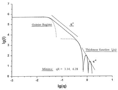
P = 4. In class we determined that all power-law scattering laws can be obtained by decomposing a structure into domains of size r and considering that  $I(q) \sim N(r) (V(r))^2$  where N(r) refers to the number of domains of size r, V(r) refers to the volume of one of these domains, and r = R/q where R is a dimensionless size that is fixed at R = 1 for the decomposition.
