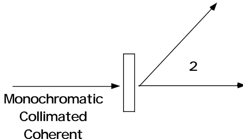
Bragg's law requires monochromatic light in order to fix  $\lambda$ , a collimated beam in order to fix the angle, and coherent radiation to have coherent interference between the waves. The coherence length must be larger than the size observed, i.e.  $d$ .
