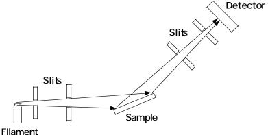
The smallest spot that can be imaged is the filament size as viewed from the sample. This limits the useful angle resolution at the dectector so determines the distance of the arm.
