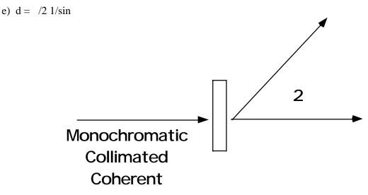
Bragg's law requires monochromatic light in order to fix , a collimated beam in order to fix the angle, and coherent radiation to have coherent interference between the waves. The coherence length must be larger than the size observed, i.e. d.
