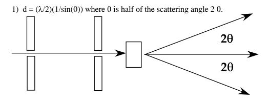
2) Collimated means that the component beams all travel in the same direction. A halogen lamp has divergent beams meaning that the beams emit in directions that serve to spread out the light. Collimation is important to Bragg's Law since the angle can only be measured with precision if the beam is well collimated. Diffraction with a divergent beam is not possible.
