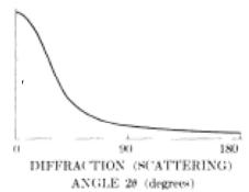
f shows a monotonic decay with 2  $\theta$  because it represents the Fourier transform of the electron density distribution function for an electron cloud which is basically a Gaussian (bell shaped) function. The Fourier transform of a Gaussian is another Gaussian which is a monotonic decay curve of the type shown above.
