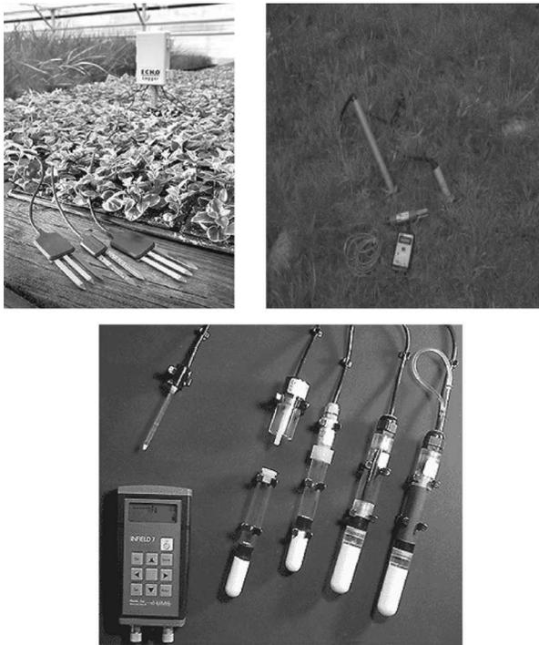
**Figure 1.13.** Electronic tensiometer.
