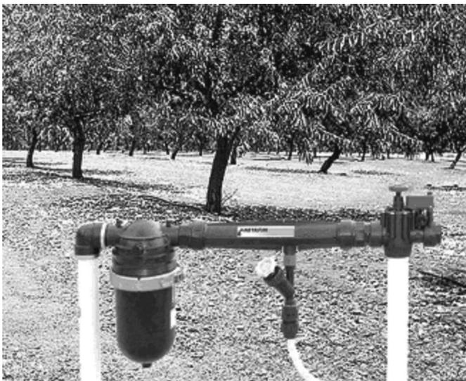
Fertilizer Injector.using Venturi system.
