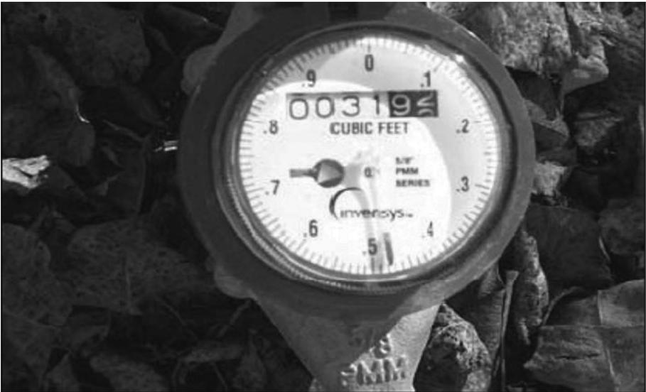
Flow meter to measure the volume of water applied.
