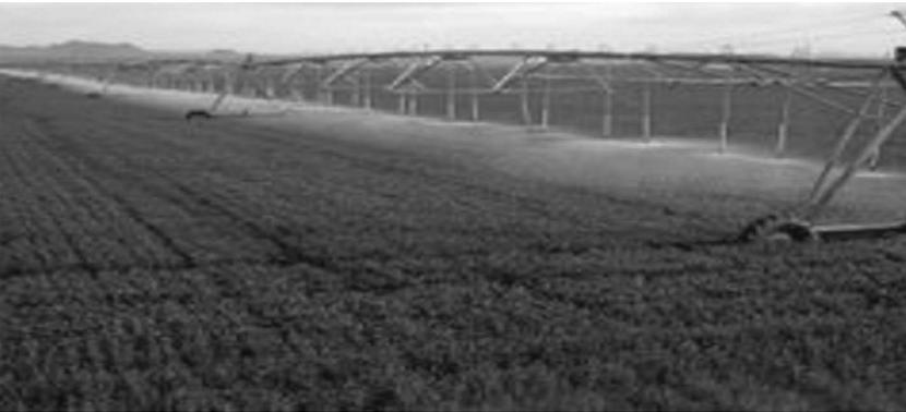
**Figure 4.11.** Center pivot with drop sprinklers.
