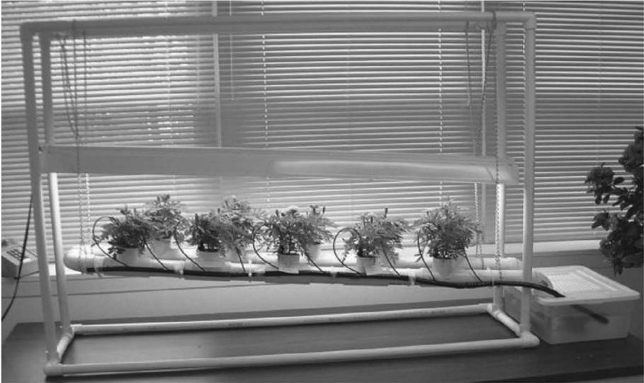
Figure 4.14. Hydroponic system.
