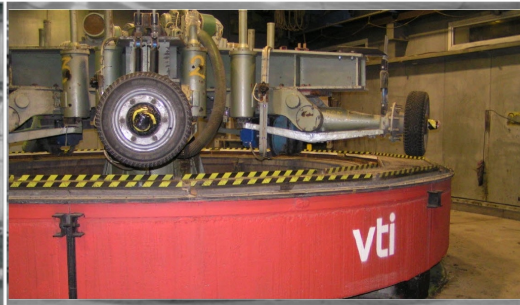
Fig. 15: Test room with the rotating axle system in the foreground and the impactor inlets in the back (left) and the VTI road simulator (right). Sources: [Left - Kupiainen et al., 2005; Right - Gustafsson et al., 2008]
