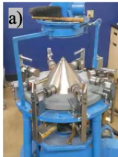
Figure 6. Instruments to be used in this study. a) Angle abrader, Akron Rubber Development Laboratory (ARDL). b) Angle Abrader wheel. c.) Rotary Drum Abrader (ARDL). d) Portable Akron Abrader.
