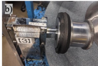
Figure 6. Instruments to be used in this study. a) Angle abrader, Akron Rubber Development Laboratory (ARDL). b) Angle Abrader wheel. c.) Rotary Drum Abrader (ARDL). d) Portable Akron Abrader.
