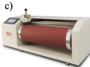
Figure 6. Instruments to be used in this study. a) Angle abrader, Akron Rubber Development Laboratory (ARDL). b) Angle Abrader wheel. c.) Rotary Drum Abrader (ARDL). d) Portable Akron Abrader.
