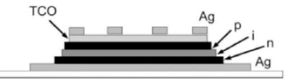
**Figure 2.6.** Printing technology using silicon nanoparticles for a solar cell. Schematic diagram of a sample printed silicon device, using nanoparticulate silicon inks. A NIP photodiode structure is shown with the silver bottom contact, N-, I-, P-type silicon layers, the printed transparent semiconducting layer (TCO), and the painted front silver, collecting grid.
