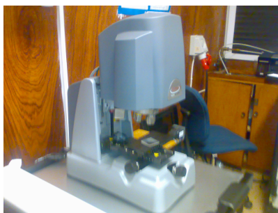
Figure 4.12. Wyko NT110 optical profiler for nanoparticle film characterization: A unique instrument on the African continent.
