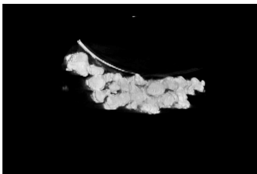
Figure 4.9. 3D tomographic reconstruction of a Silicon nanoparticle cluster by transmission electron microscopy. The large particle on the left is approximately 200nm across.
