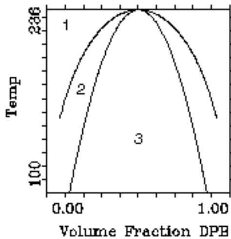
Figure 2. Upper critical solution temperature phase diagram. Regions 2 and 3 are 2-phase regimes, region 1 is the single phase regime. The line between region 2 and 1 is the cloud point curve or the binodal curve.
