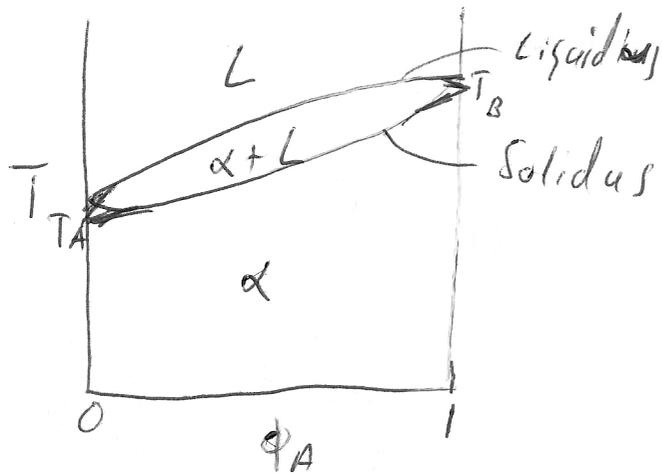
A & B have the same crystal structure and close to the same atomic size. A & B make a solid solution.
