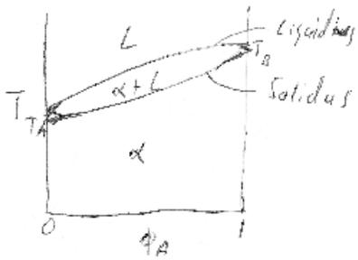
A & B have the same crystal structure and close to the same atomic size. A & B make a solid solution.
