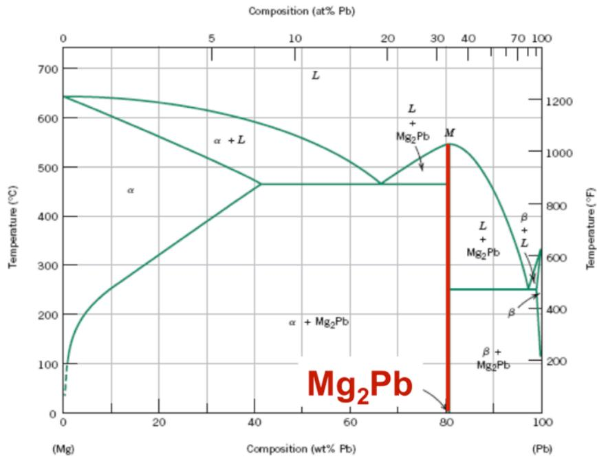
Note: intermetallic compound exists as a line - not an area – because stoichiometry (i.e. composition of a compound) is fixed.
