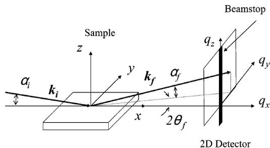
**Figure 1.** Schematic GISAXS experiment. Incident X-ray beam ( $k_i$ ) angle and scattered beam ( $k_f$ ) are  $\alpha_i$  and  $\alpha_f$  respectively. Scattering vectors  $q$  are calculated from  $(4\pi/\lambda) \sin \theta_f$ , where  $\theta_f$  is the scattering half angle and  $\lambda$  is the wavelength of the X-rays.
