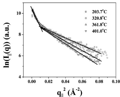
**Figure 2.** Data are shown for horizontal slices at selected temperatures and fits are derived from Guinier analysis. The low  $q$  section, which does not change with temperature, is likely to result from scattering of the substrate.
