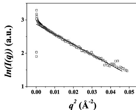
**Figure 3.** Data for Guinier analysis of vertical slices for all temperatures. Only one region is found that results from the height of the clusters on the surface.
