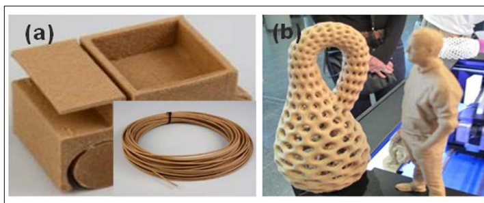
Fig. 7 - Application of wood fibre in 3D printing: (a) Laywoo-D3™ [36]; (b) WoodFill™ developed by ColorFabb [37].
