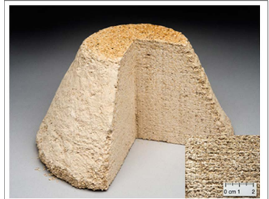
Fig. 9 - Truncated cone generated by 3D printing with spruce chips and gypsum, cut open to show the inner texture [39].
