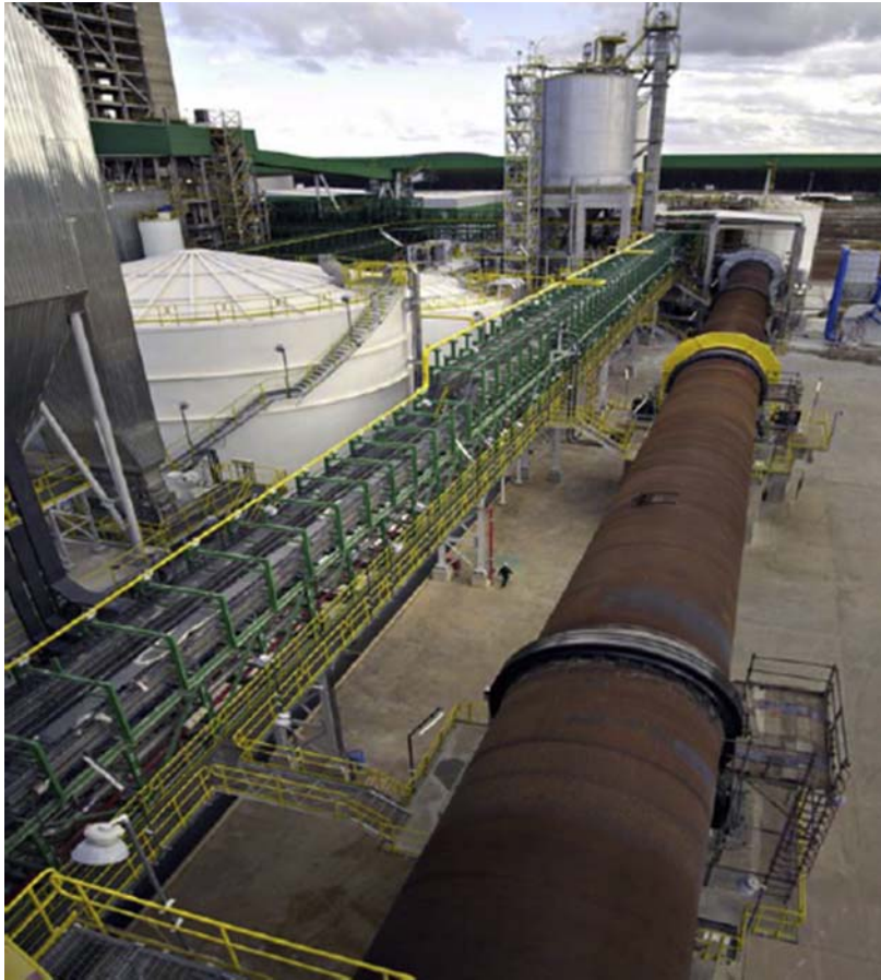
FIGURE 17.18 Andritz's lime reurning kiln system ensures reliable and energy efficient production of high-quality lime for the recausticizing operation. Courtesy: Andritz
